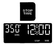
6. Use the Hour and Minute pads to set the desired stop time. Push the "up" (▲) or "down" (▼) pad(s) until the correct time shows on the display.
