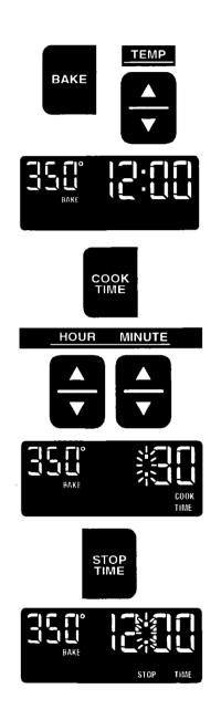
Use the Hour and Minute pads to set the desired stop time. Push the "up" (▲) or "down" (▼) pad(s) until the correct time shows on the display.
