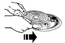
When the terminal is pushed into the receptacle as far as it will go, push down the edge of the surface unit opposite the receptacle. The element hold-down clip will keep the surface unit from moving around.
